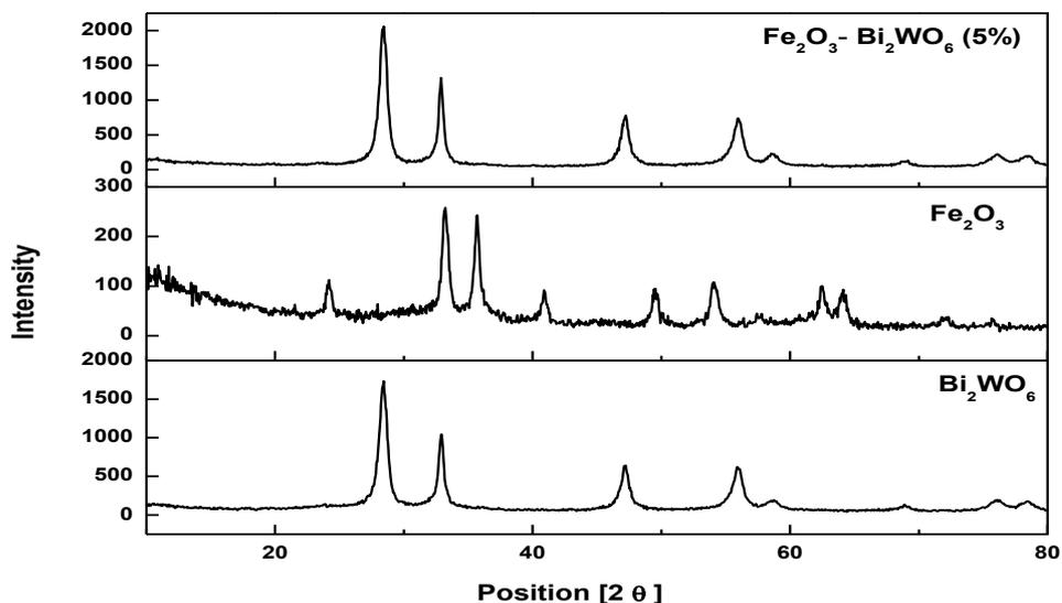
Figure 2. The XRD patterns of the catalysts prepared
