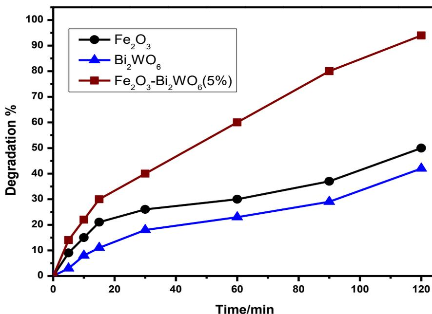
**Figure 4.** Photocatalytic removal of Dox with Fe<sub>2</sub>O<sub>3</sub>, Bi<sub>2</sub>WO<sub>6</sub> and Fe<sub>2</sub>O<sub>3</sub>-Bi<sub>2</sub>WO<sub>6</sub> composites as photocatalyst in the presence of H<sub>2</sub>O<sub>2</sub> (5 %)
