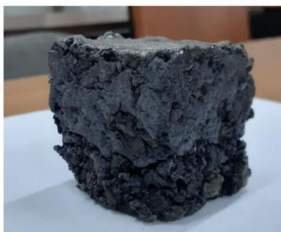
**Figure 1.** The appearance of the resulting coal briquette
