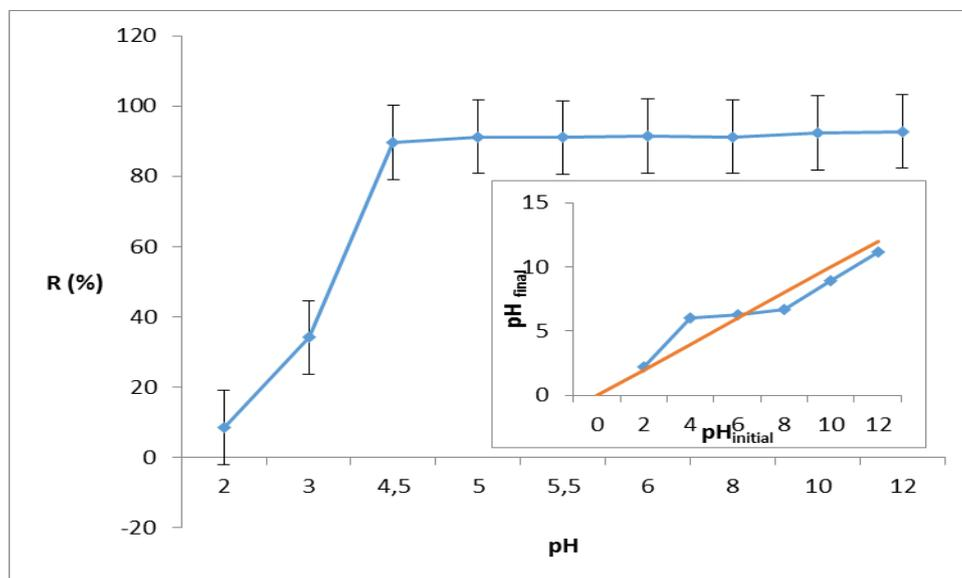
**Figure 5.** Effect of medium pH on the adsorption rate of copper by CSS
