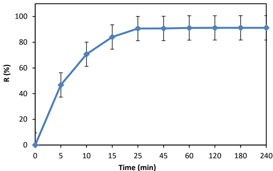
**Figure 3.** Effect of contact time on the adsorption rate of MB by CSS
