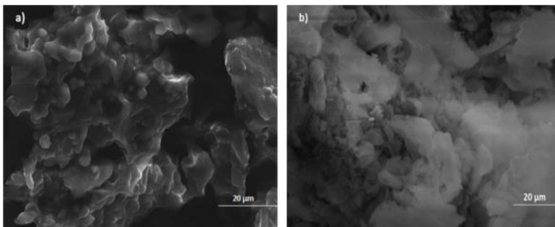
**Figure 2.** SEM micrographs of CSS before (a) and after (b) adsorption of MB
