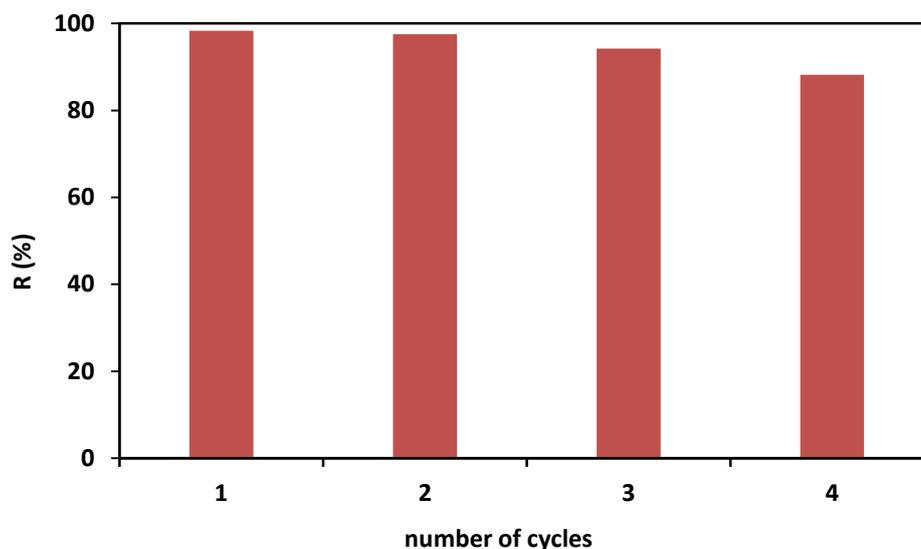
Figure 9. Four (Adsorption / desorption) cycles using 0.1M HCl
