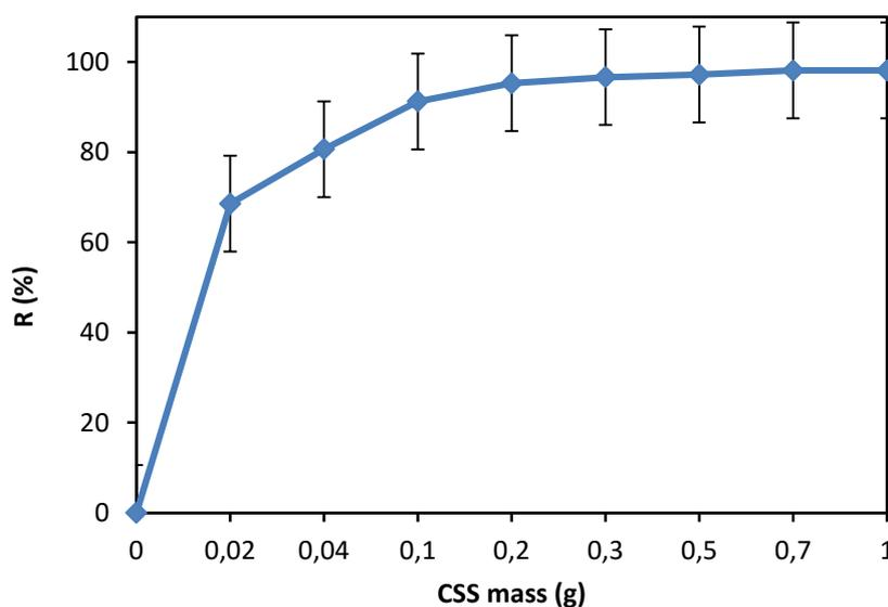
**Figure 4.** Effect of adsorbent mass on the adsorption rate
