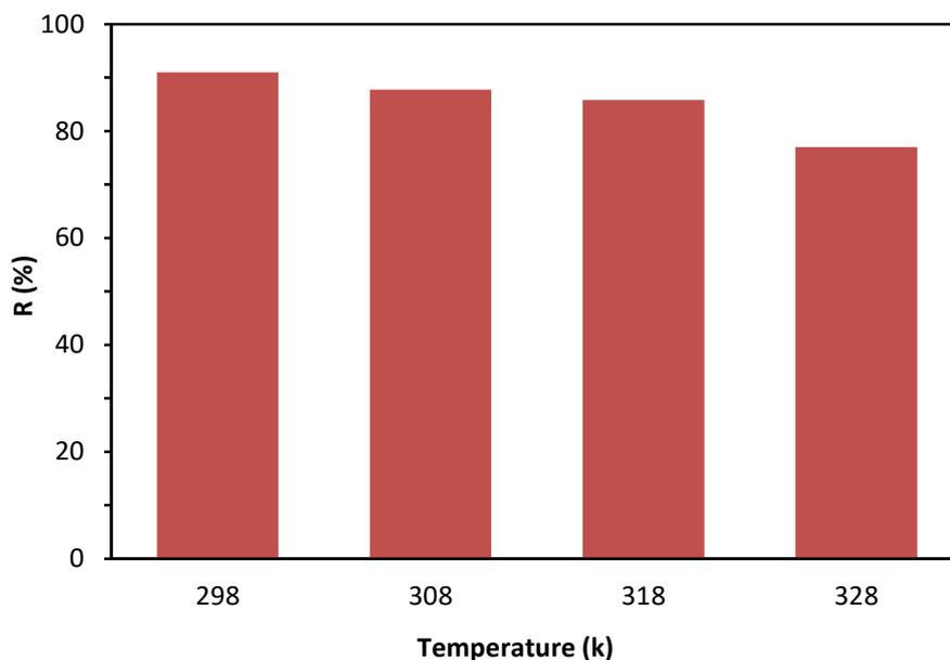
**Figure 7.** Effect of temperature on the adsorption of MB by CSS
