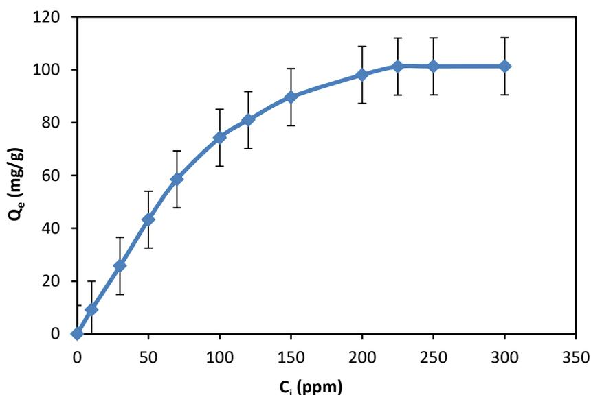
**Figure 6.** Effect of initial concentration of MB on the amount of adsorption
