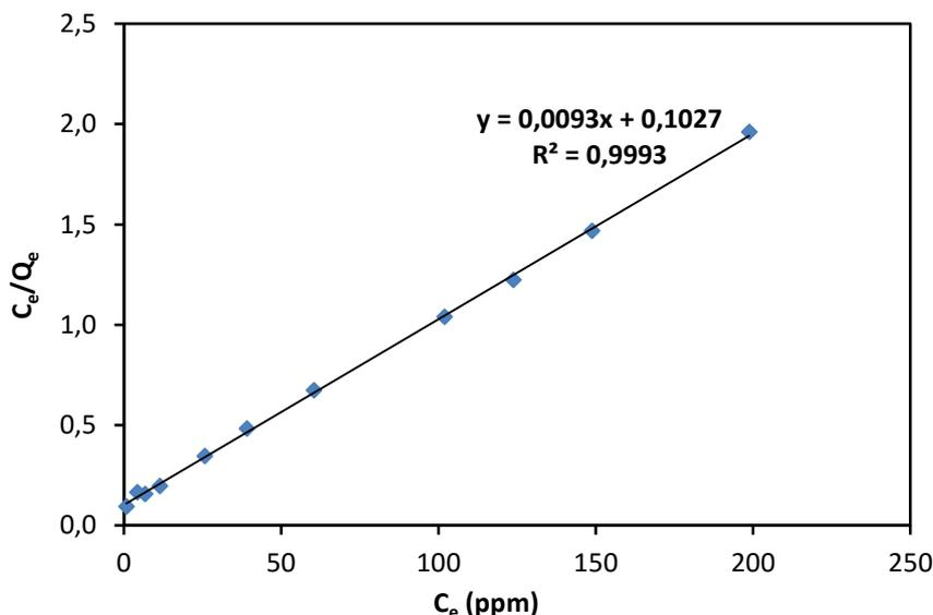
Figure 12. Langmuir isotherm model
