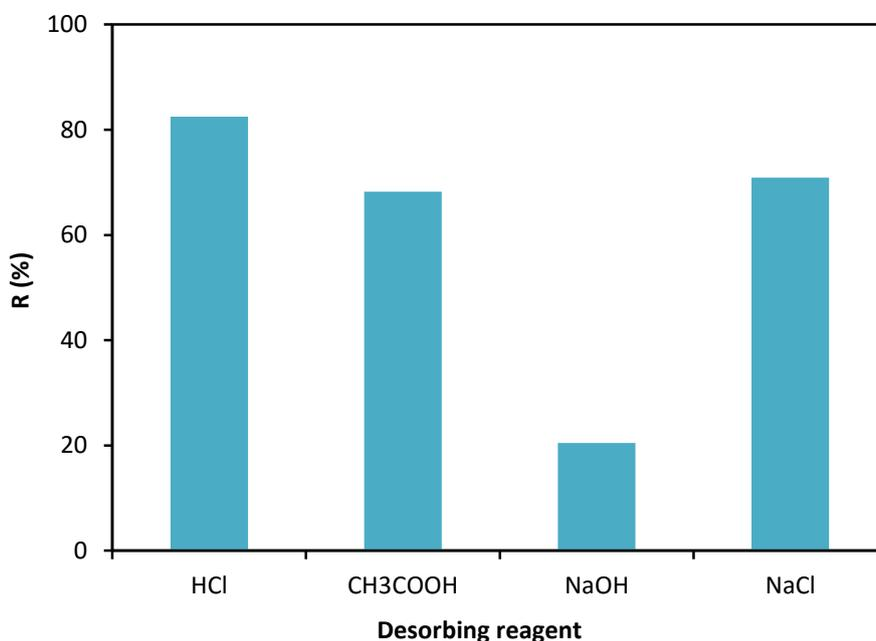
**Figure 8.** Desorption of MB dye from CSS using different desorbing reagents
