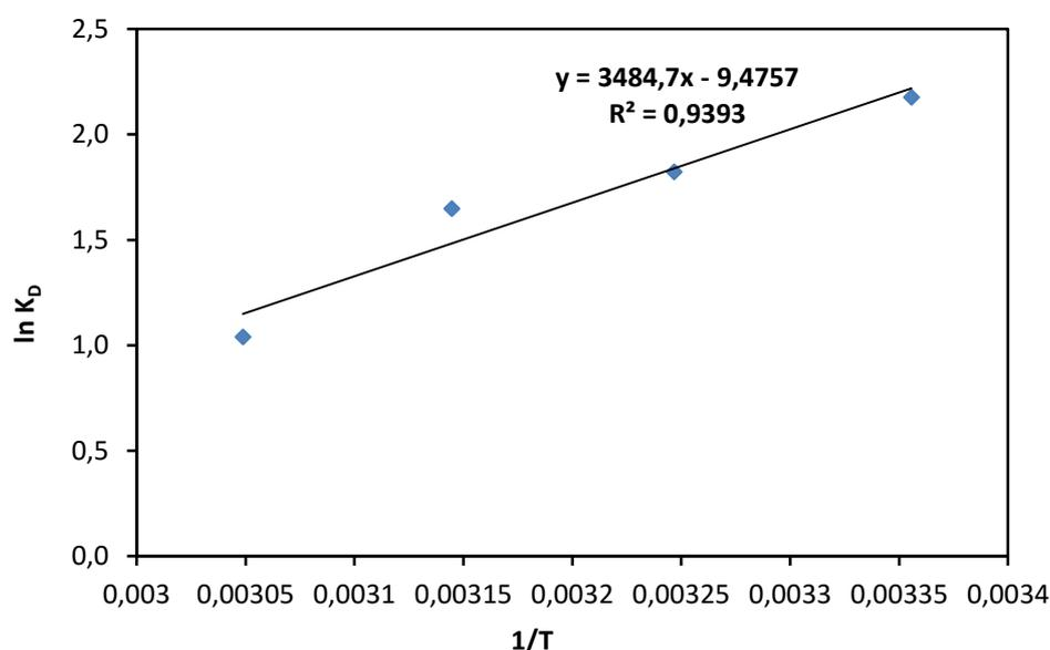
**Figure 15.** Van'tHoff curve corresponding to the adsorption of MB by CSS
