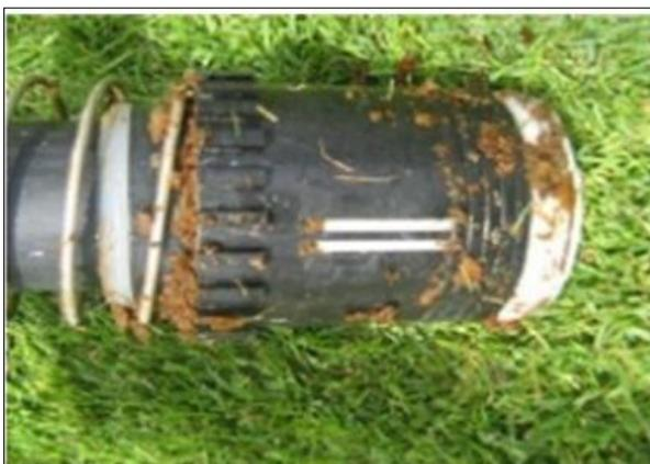
**Figure 2.** Sprinkler clogged by the scale
