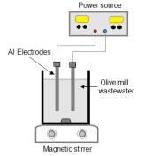
Figure 1. Schematic of the electrocoagulation cell
