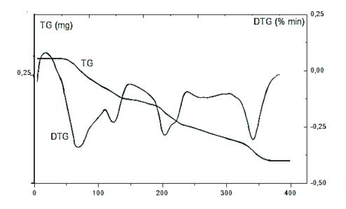
Figure 5.TGA (TG and DTG) curve of  $MnSr_2(P_3O_9)_2, 4H_2O$  at rising temperature (5°C min<sup>-1</sup> / P = 1 atm)
