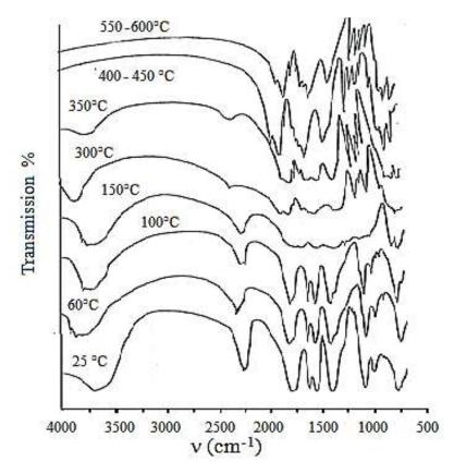
Figure 4. IR Absorption Spectra of MnSr<sub>2</sub> (P<sub>3</sub>O<sub>9</sub>)<sub>2</sub>.4H<sub>2</sub>O and its thermal dehydration products at atmospheric pressure
