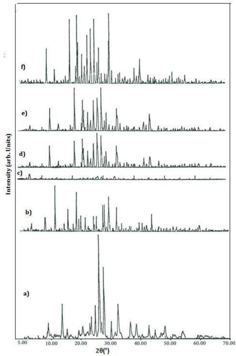
**Figure 3.** X-ray diffractograms of  $MnSr_2(P_3O_9)_2.4H_2O$  (a) and its dehydration products at atmospheric pressure: (b)100°C, 200°C (d) evolution to the mixture  $(2\gamma[Sr(PO_3)_2]_{\infty}+[Mn(PO_3)_2]_{\infty})$ , (e) mixture  $(2\gamma[Sr(PO_3)_2]_{\infty}+[Mn(PO_3)_2]_{\infty})$  and (f) mixture  $([Mn(PO_3)_2]+2\beta[Sr(PO_3)_2])$
