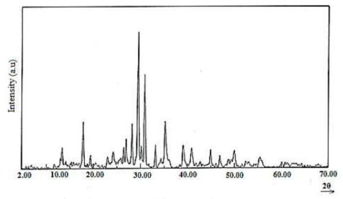
Figure 1. X-ray powder diffractogram of MnSr<sub>2</sub>(P<sub>3</sub>O<sub>9</sub>)<sub>2</sub>.4H<sub>2</sub>O
