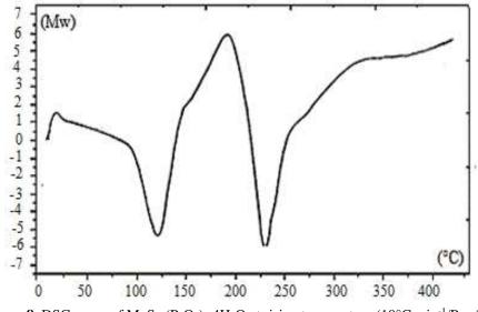
Figure 8. DSC curve of  $MnSr_2(P_3O_9)_{2,4}H_2O$  at rising temperature (10°C min<sup>-1</sup>/P = 1 atm)
