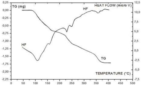
Figure 6. TGA and DTA curves of  $MnSr_2(P_3O_9)_2.4H_2O$ , at rising temperature (5°C min<sup>-1</sup> / P =1 atm)
