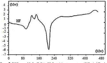
**Figure7.** DSC curve MnSr<sub>2</sub>(P<sub>3</sub>O<sub>9</sub>)<sub>2</sub>,4H<sub>2</sub>O at rising temperature (5°C min<sup>-1</sup>/P = 1atm)
