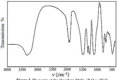
Figure 2. IR spectra of the phosphate MnSr<sub>2</sub> (P<sub>3</sub>O<sub>9</sub>)<sub>2</sub>.4H<sub>2</sub>O
