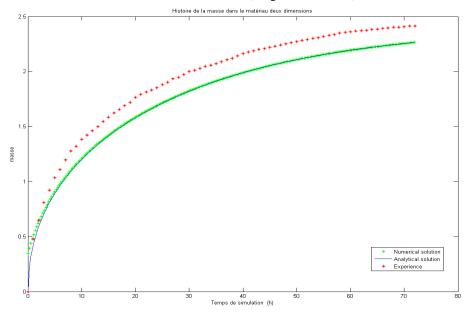
Figure 7. The amount of water transferred to the sample as a function of the simulation time in the twodimensional direction (longitudinal-tangential)
