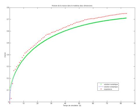
Figure 8. The amount of water transferred to the sample as a function of the simulation time in the twodimensional direction (radial-tangential).
