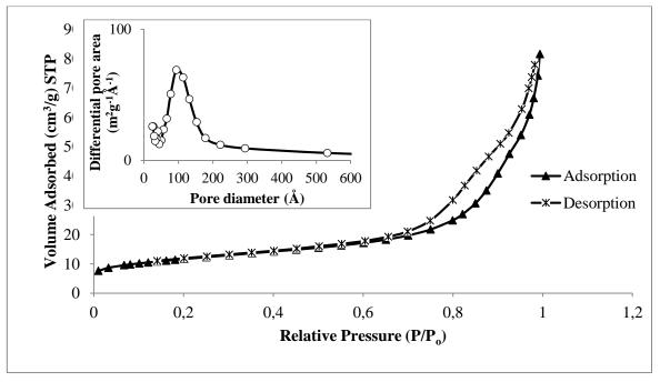
Figure 1. Fresh Zn-Cr (10:1) nitrogen adsorption and desorption isotherm.
