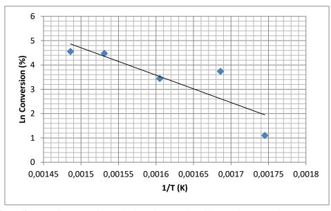
**Figure 4.** Arrhenius plots of ketonisation of pentanoic acid over Zinc-Chromium (10:1) oxide (  $300-400^{\circ}$ C, 1 bar pressure, 0.2 g catalyst, 20 mL min<sup>-1</sup> N<sub>2</sub> flow rate and 2 vol % of pentanoic acid).
