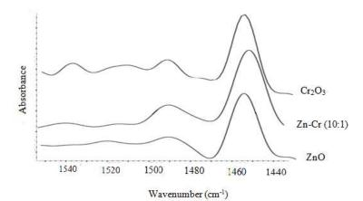
Figure 3 DRIFT spectra of pyridine adsorption for zinc-chromium catalysts.
