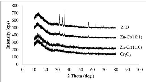
Figure 2. X-ray diffraction for the zinc-chromium catalyst.
