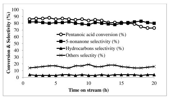
Figure 5. Ketonisation of pentanoic acid on Zinc-Chromium (10:1) oxide ( $350^{\circ}$ C, 1 bar pressure, 0.2 g catalyst, 2 vol % of acid, 20 mL min<sup>-1</sup> N<sub>2</sub> flow rate and 4.0 h g mol<sup>-1</sup> space-time).
