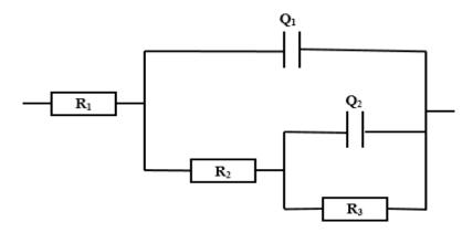
Figure 4. Equivalent circuit model for electrochemical impedance measurements.
