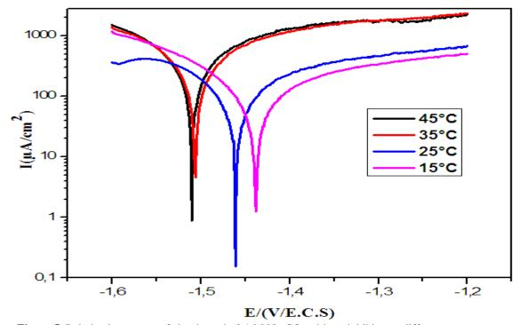
Figure 5. Polarization curves of aluminum in 0.1 M Na<sub>2</sub>CO<sub>3</sub> without inhibitor at different temperatures.
