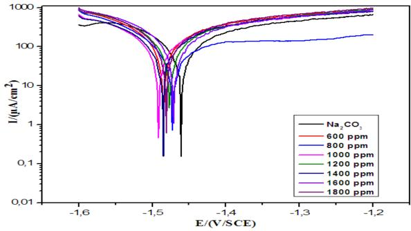
Figure 2. Polarization curves of aluminum in 0.1 M Na<sub>2</sub>CO<sub>3</sub> with and without inhibitor at  $25 \pm 0.1$  ° C.
