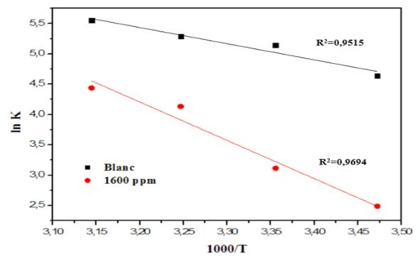
Figure 9. Arrhenius Curves of aluminum in 0.1 M Na<sub>2</sub>CO<sub>3</sub> with and without inhibitor
