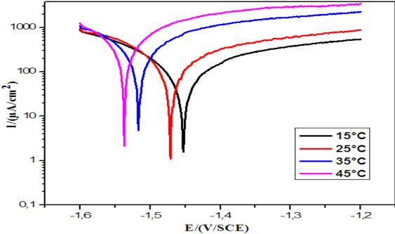
**Figure 6.** Polarization curves of aluminum in 0.1 M Na<sub>2</sub>CO<sub>3</sub> with the presence of 1600 ppm of the inhibitor at different temperatures.
