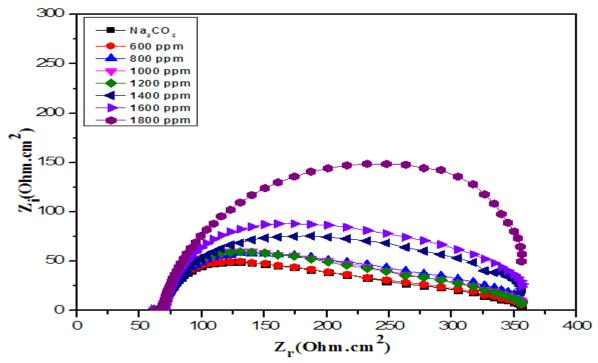
Figure 3. Nyquist curves of aluminum in Na<sub>2</sub>CO<sub>3</sub> with and without addition of the inhibitor at 25  $\pm$  0.1  $^{\circ}$  C.
