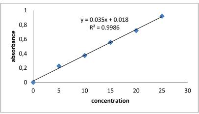
Figure 3. Calibration curve of BF
