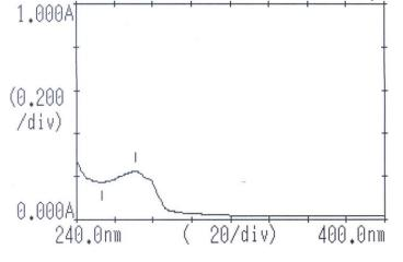
Figure 2. UV spectrum of BF aqueous solution (271nm; 5µg/ml)
