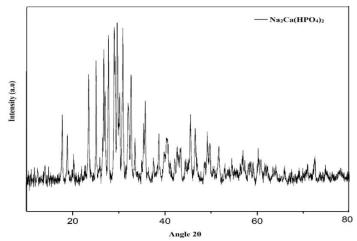
Figure 2. XRD Analysis Spectrum of Na<sub>2</sub>Ca(HPO<sub>4</sub>)<sub>2</sub>.
