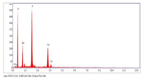
Figure 5. EDAX analysis of the chemical constituents of Na<sub>2</sub>Ca(HPO<sub>4</sub>)<sub>2</sub>.
