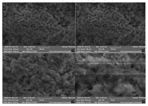
**Figure 3.** Images of Na<sub>2</sub>Ca(HPO<sub>4</sub>)<sub>2</sub> taken by SEM.
