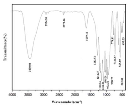
Figure 4. Infrared Spectra of Na<sub>2</sub>Ca(HPO<sub>4</sub>)<sub>2</sub>.
