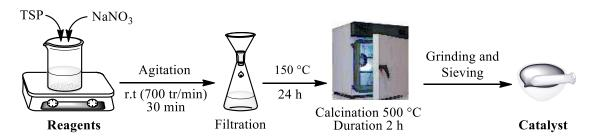
Figure 1. Different steps of Na<sub>2</sub>Ca(HPO<sub>4</sub>)<sub>2</sub> preparation.
