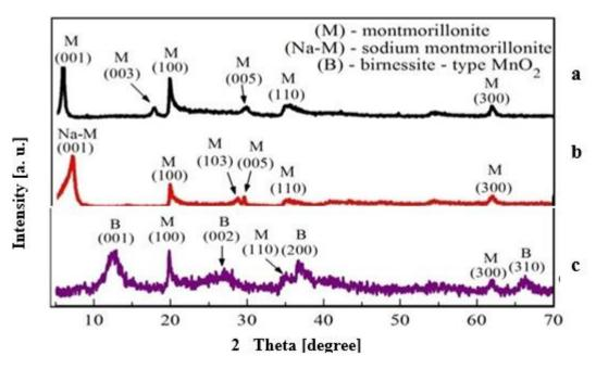
Figure 1. X-ray diffraction (XRD) patterns of the B (a), NaB (b), and Mn-NaB (c)
