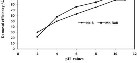
Figure 3. pH influence on the removal of radium from uranium effluent
