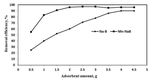
Figure 4. Effect of adsorbent amount on radium removal
