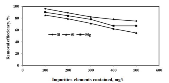
Figure 5. Interfering elements influence on the removal of radium efficiency at pH 1.8
