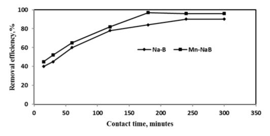
Figure 6. Effect of contact time on radium removal from uranium effluent at pH 10
