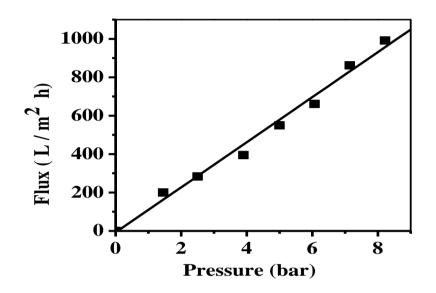
Figure 4. Water flux through the membrane ACZA-60 vs. working pressure
