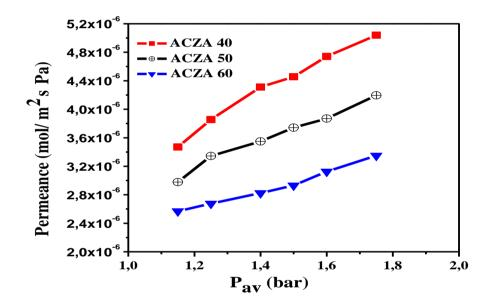
Figure 3. N<sub>2</sub> permeances of as-synthesized NaA zeolite membranes
