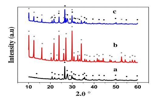
**Figure 1.** XRD patterns of: (a) substrate, (b) NaA zeolite crystals and (c) as-synthesized membrane (synthesis temperature of 60 °C), obtained after seeding the clay support; (•) support (•) NaA zeolite
