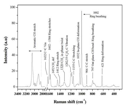
Figure 2. Assignments of the characteristic Raman peaks in polystyrene
