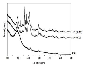
**Figure 6.** XRD patterns for the PSt (0) and HP (0,1& 0,25) **Table 2.** XRD values for the HP crystallite.
