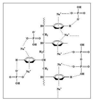
Scheme 1. Possible interactions between the polymer matrix and sodium phosphates
