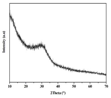
Figure 3. XRD spectra of NaPO<sub>3</sub>
