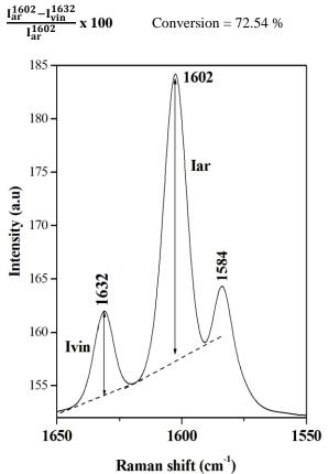
Figure 1. Determination of I<sub>ar</sub> and I<sub>vin</sub> intensities by Raman spectroscopy
