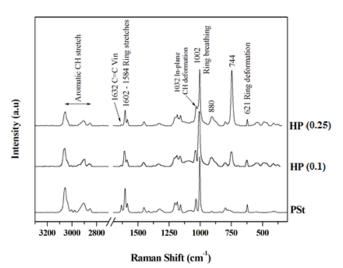
**Figure 7.** Raman spectrums of PSt and HP (0.1; 0.25) from 3300 to 300 cm<sup>-1</sup>at room temperature
