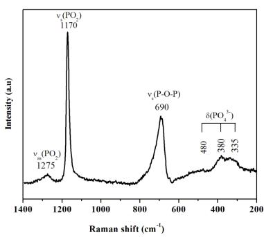
Figure 4. Assignments of the characteristic Raman peaks in NaPO<sub>3</sub>
