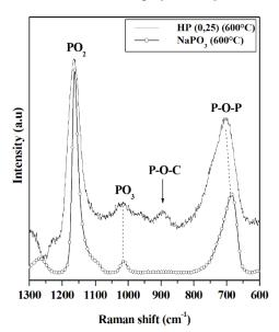
**Figure 11.** Raman spectra of the pyrolysis residues of NaPO<sub>3</sub> and HP (0.25) at 600 °C
