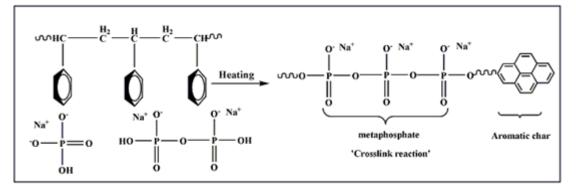
Scheme 2. Degradation process of (PSt/ Phosphate) system
