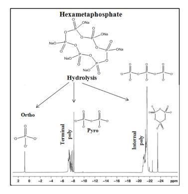
Figure 5. <sup>31</sup>P liquid NMR spectrum of hydrolyzed commercial polyphosphate NaPO<sub>3</sub>
