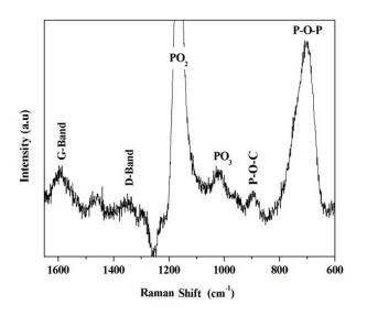
**Figure 10.** Raman spectra of the pyrolysis residue of HP (0.25) in region 1650–600 cm<sup>-1</sup>at 600 °C
