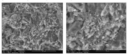
Figure 8. SEM microphotos of scale at sprinklers
