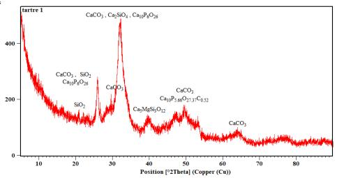
Figure 5. X-ray diffractogram of the scale taken from the sprinklers
