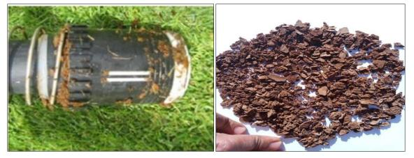
Figure 2. Sprinkler clogged by the scale
