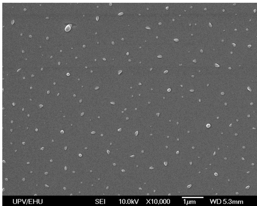
**Figure 3.** SEM photomicrography of the nanogels.
